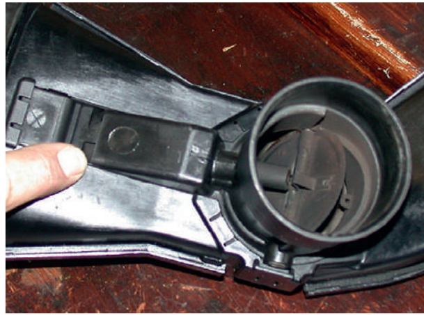
Figure 2.192 Warm-air control (vacuum type)
